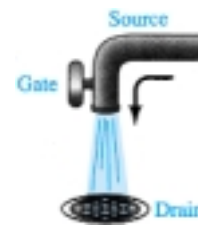
Figure 5.3 Water analogy for the JFET control mechanism.
