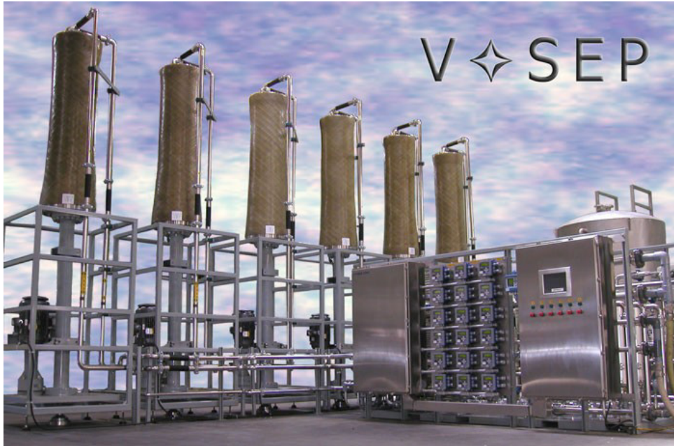
Fig 23. Industrial VSEP modules with 150 m 2 of membranes
