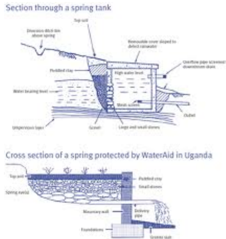
Figure 4.3. Example of Spring Protection from a WaterAid project in Uganda [15]
