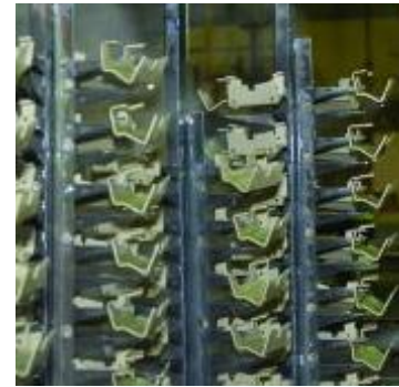
(b) Electroplated parts on a rack are moved from one bath to the next.
