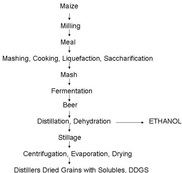
Fig 4.5 Ethanol production from maize (dry-grind process)
