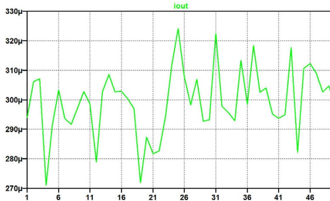
Figure 6.25: Output current variation for the 50 simulations with random values for the threshold voltage of M_2 .
