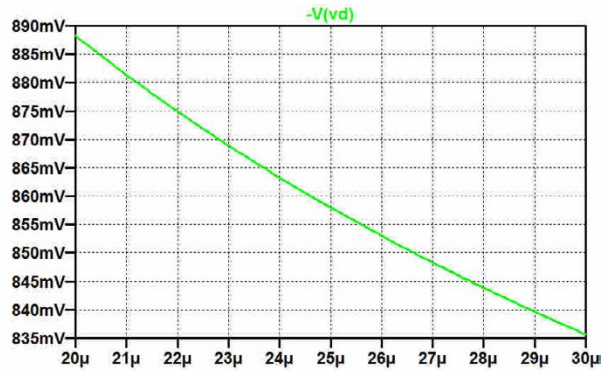
Figure 5.14: Simulation showing |V_{GS}| versus W for a PMOS transistor with L = 1 \mu\text{m} and I_D = 30 \mu\text{A} using the BSIM3 transistor model.
