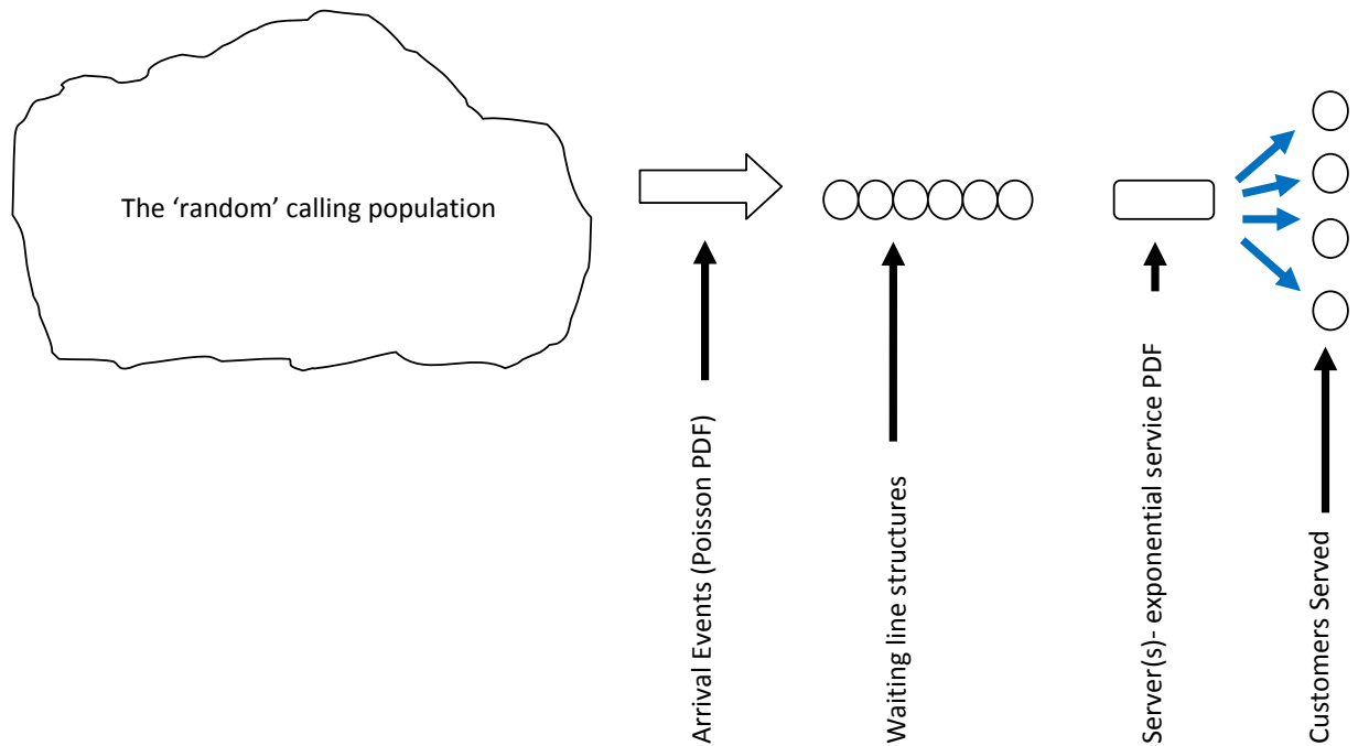
Figure 4.4 – Basic components of a Queue
