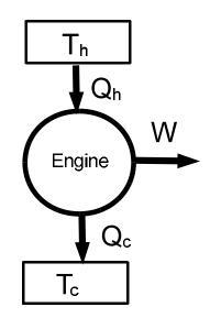
We conclude that a heat engine must operate between two heat baths at temperatures  $T_h$  and  $T_c$ , respectively. Heat is removed from the bath at the higher temperature  $T_h$  and heat is expelled at the lower temperature  $T_c$ . Conservation of energy gives  $Q_h = W + Q_c$  so that
