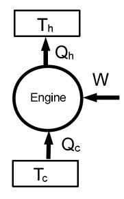
A heat pump can be used for heating. The engine requires the input of work [e.g., by plugging it in an electric outlet] and removes heat  $Q_c$  from cold reservoir [outside] and delivers heat  $Q_h$  into hot reservoir [inside the house]:  $Q_c + W = Q_h$ . Coefficient of performance is defined as the ratio of the gain
