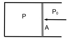
The pressure inside and outside a piston is P and  $P_0 < P$ , respectively. If the cross-sectional area of the piston is A, a force  $F = (P - P_0) \cdot A$  must be applied to move the piston to the left.
