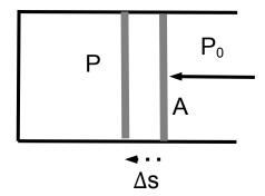
If the piston is displaced by  $\Delta s$ , work is done on the gas:  $W = F \cdot \Delta s$ . We find  $W = (PA) \cdot \Delta s = P(A \cdot \Delta s) = -P\Delta V$ , where we used  $A\Delta s = -\Delta s$  [negative, because the volume of the gas *decreases*]. This yields an alternative definition of pressure
