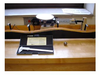
**Example 2**: A steelball with mass m = 0.44 kg and radius r = 1.0 cm moves along a roller coaster. Seven photogates are placed along the track at different heights  $h_i$  from the base of the track; we measure the time intervals  $\Delta t_i$  for the steel ball to pass through each photogate,
