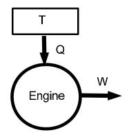
The engine returns to the same 'state' after one cycle [represented by the circle]. Heat is transferred at the temperature T and the output is in the form of work W. This engine would give a net loss of entropy  $\Delta S = -Q/T$ , and thus would violate the second law of thermodynamics. We conclude that not all heat converted into work, and that the engine must expel heat as exhaust.
