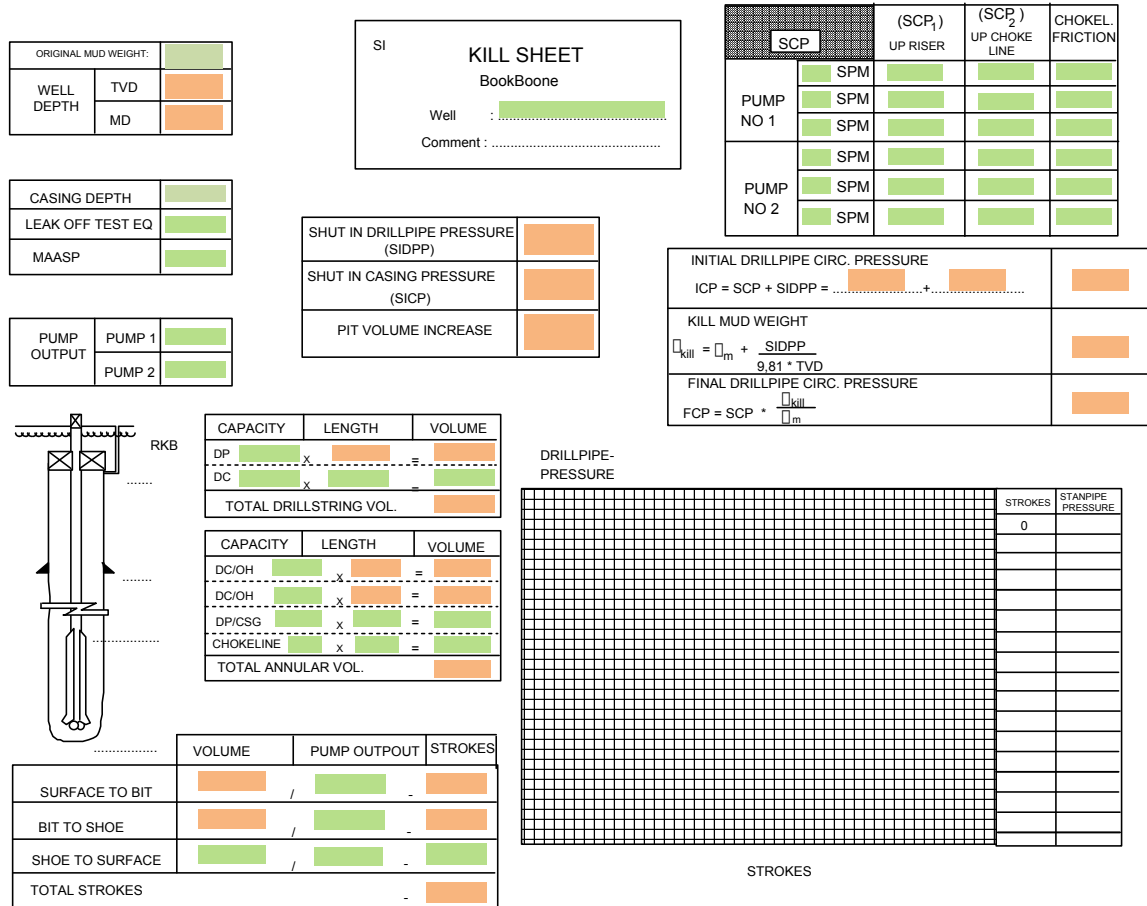
Figure 4-13: An example of Kill sheet. Green boxes indicate information known before a kick is taken. They must be updated at least every shift (every 12 hours). Red boxes represent information that is known after shut-in.
