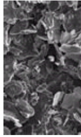
Figure 5-18: Natural Crystalline Flake Graphite is also used as Carbon Brushes. As pack and seal material it comes in the size of 5-425 microns.
