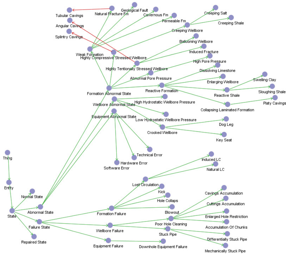
Figure 8-22: Errors during oil well drilling, grouped with respect to location of where they emerge. If these errors are detected at the surface location we call them indicative symptoms of failures.
