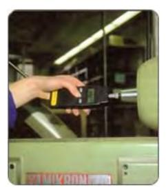
Figure 5.9 Digital Tachometer Courtesy of http://www.vaiseshika.com/
