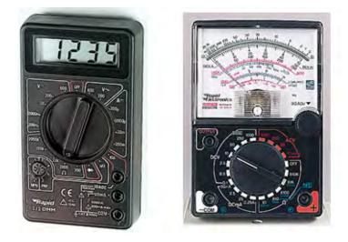
Figure 5.3 Digital and Analog Multimeters Courtesy of <u>http://www.kpsec.freeuk.com/multimtr.htm</u>
