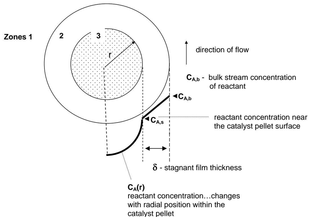
**Figure 6.1** Three contiguous zones are defined, to help formulate reaction rate expressions in catalyst beds: (1) bulk fluid phase, (2) stagnant film surrounding the catalyst pellet, and, (3) the catalyst pellet.
