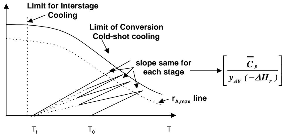
**Figure 4.9** A “cold-shot” cooled reactor system consists of a series of adiabatic catalyst chambers. In each of the reactor stages, the temperature rises from inlet to outlet. A cold shot of initial feed material is introduced between stages to cool the reaction stream to a pre-determined temperature.
