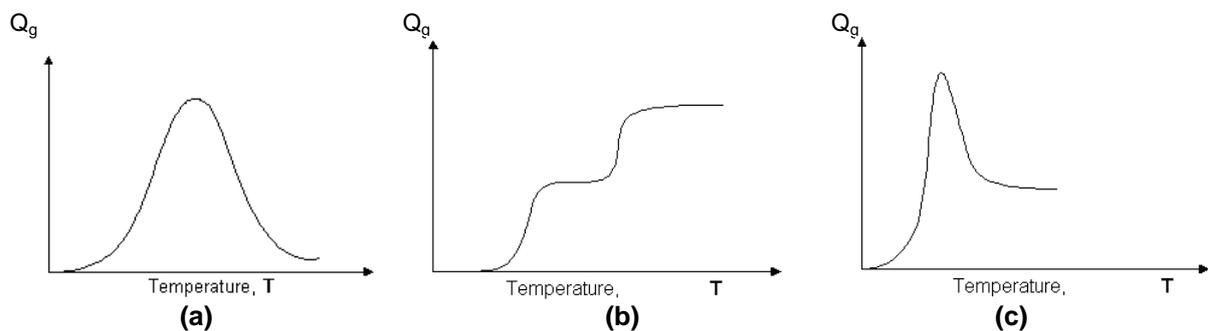
**Figure 3.3** The qualitative shape of  $Q_g$ , the heat generation term, for (a) a reversible reaction, (b) a pair of consecutive exothermic reactions and (c) for two consecutive reactions, where the first is exothermic and the second is endothermic.
