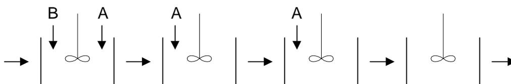
**Figure 4b** Keeping the reagent concentration low in CSTRs in series, by small additions of reagent further downstream
