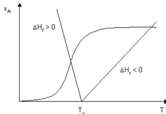
**Figure 3.5** The material and energy balance lines for a non-isothermal CSTR. The intersections indicate the position of the simultaneous solution.
