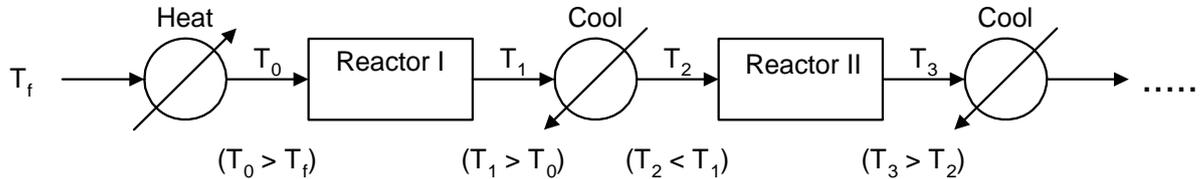
**Figure 4.6** Schematic diagram of two reactors in series. The first heat exchanger heats the feed stream from  $T_f$  to the reactor inlet temperature  $T_0$ . After “Reactor I” the temperature  $T_1$  is dropped to  $T_2$  before entering “Reactor II”.
