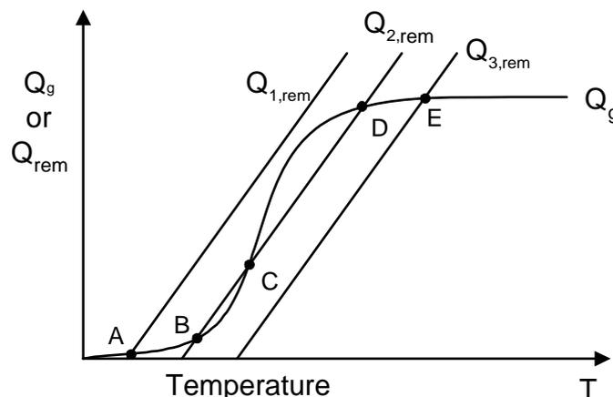
**Figure 3.2** Comparing the heat generation,  $Q_g$  and heat removal  $Q_{rem}$  terms in the CSTR energy balance equation (Eq. 3.23).
