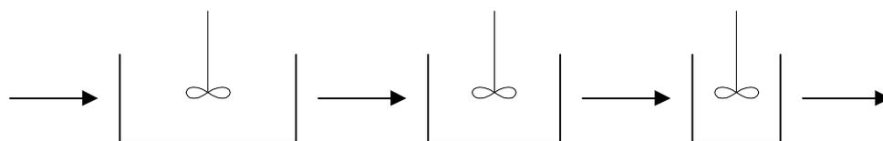
**Figure 3** Where the desired reaction is of the lower order, the concentration of reagent should be kept as low as possible. The use of CSTR's has advantages over the use of batch or tubular reactors. Only a small number of tanks in series is used and the first is made relatively large.
