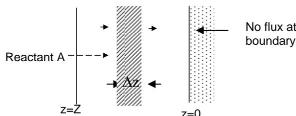
**Figure 6.5** Schematic diagram of flat-plate catalyst pellet with volume element  $\alpha \Delta z$ ;  $\alpha$  is the surface area.
