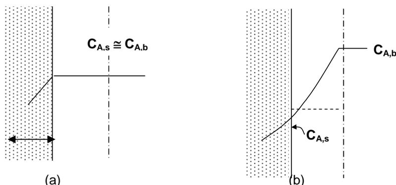
**Figure 6.3** (a) When the process is controlled kinetically, i.e. when reaction is slower than diffusion, the concentration gradient across the external stagnant film tends to flatten. (b) When external diffusion is slower than chemical reaction, a concentration gradient is set up across the stagnant film. This is called external diffusion control.
