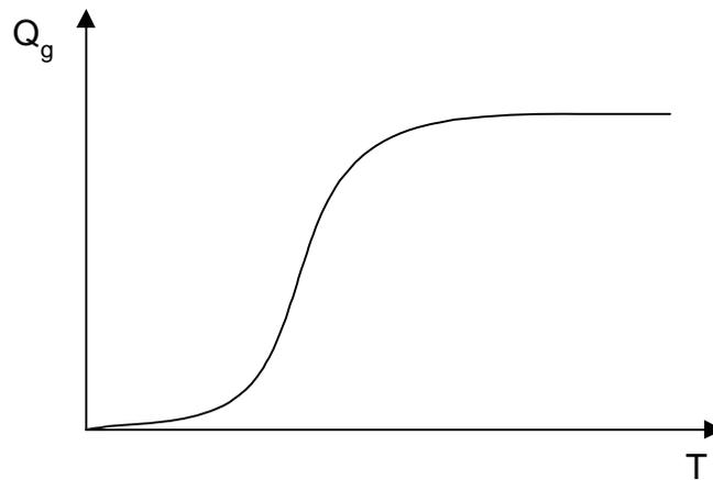
**Figure 3.1** The form of heat generation term for a CSTR (Eq. 3.26) as a function of increasing temperature. At high values of  $T$ ,  $k$  is so large that virtually no unreacted reagent remains in the exit stream.
