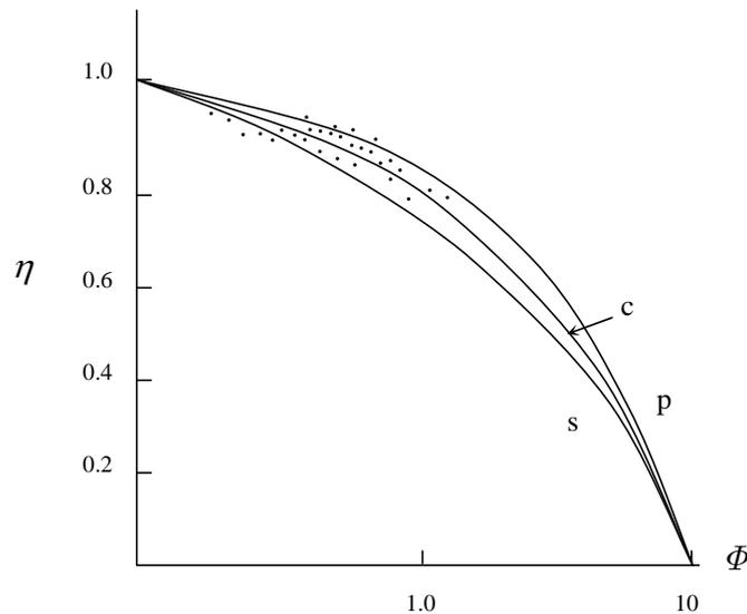
**Figure 6.8** Isothermal effectiveness factor for three geometries plotted against the generalized Thiele modulus. The dots indicate some of the empirical findings. Note that the scatter is of the same order of magnitude as the divergence between the lines.
