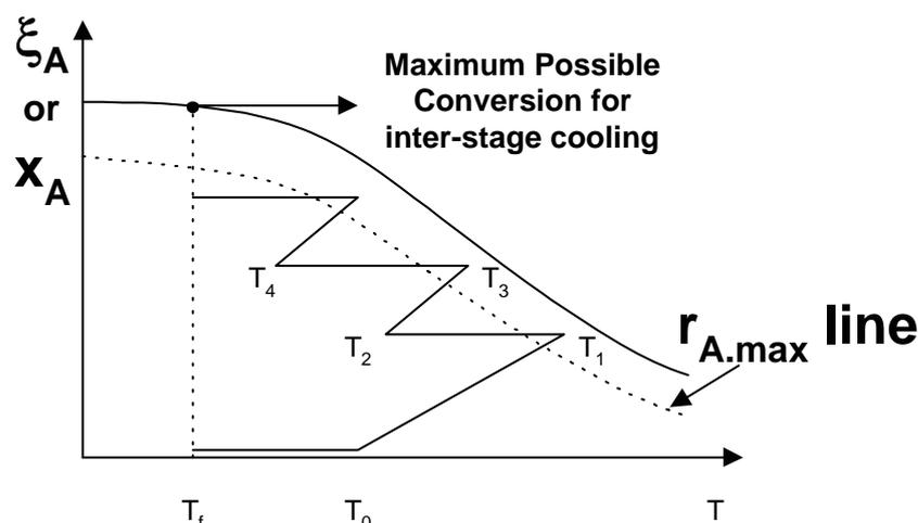
**Figure 4.7** An inter-stage cooled reactor system consists of a series of adiabatic catalyst chambers. In each of the reactor stages, the temperature rises from inlet to outlet. Then an interstage cooler cools the reaction stream to a pre-determined temperature.
